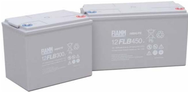
**HIGHLITE** batteries have been specifically designed to give optimal standby performance for applications requiring high-rate discharges. FIAMM **HIGHLITE** batteries are Valve Regulated Maintenance Free types with the electrolyte absorbed in microporous glass fiber separators. **HIGHLITE** batteries can be installed in cabinets or on racks and minimum installation space is required due to the high energy density characteristics of this range.
